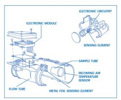
moving parts. Instead, they use a heated sensing element to measure air flow.
